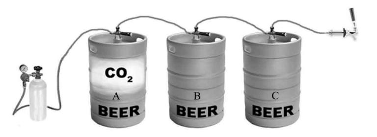
When introducing new filled kegs to the line always remove partially filled keg and move it back to position "A" nearest the air distributor.
